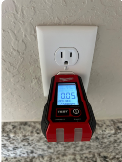
Bathroom 2 GFCI Trips and Resets
