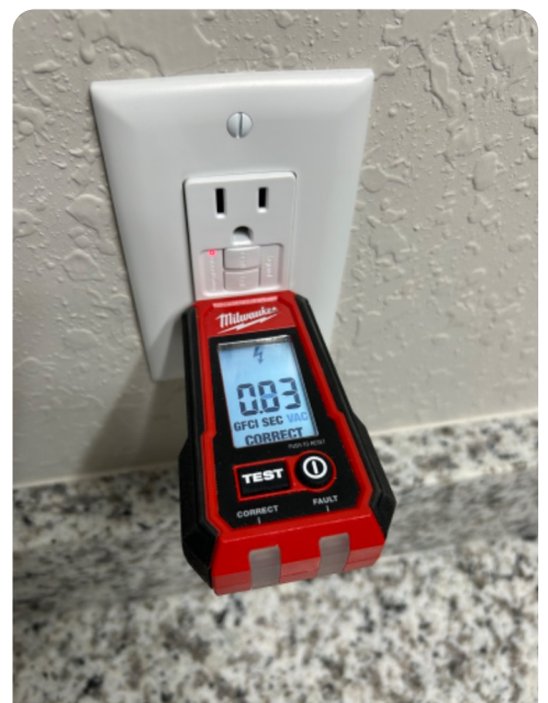
Master Bathroom GFCI Trips and Resets
